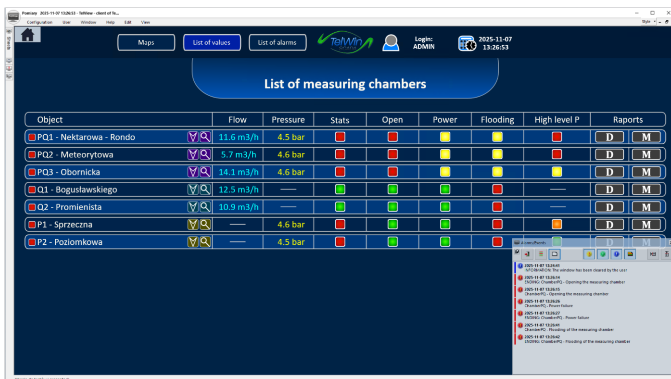
FIGURE 4 TelVIEW - SAMPLE DIAGRAM WITH ALARM LIST
